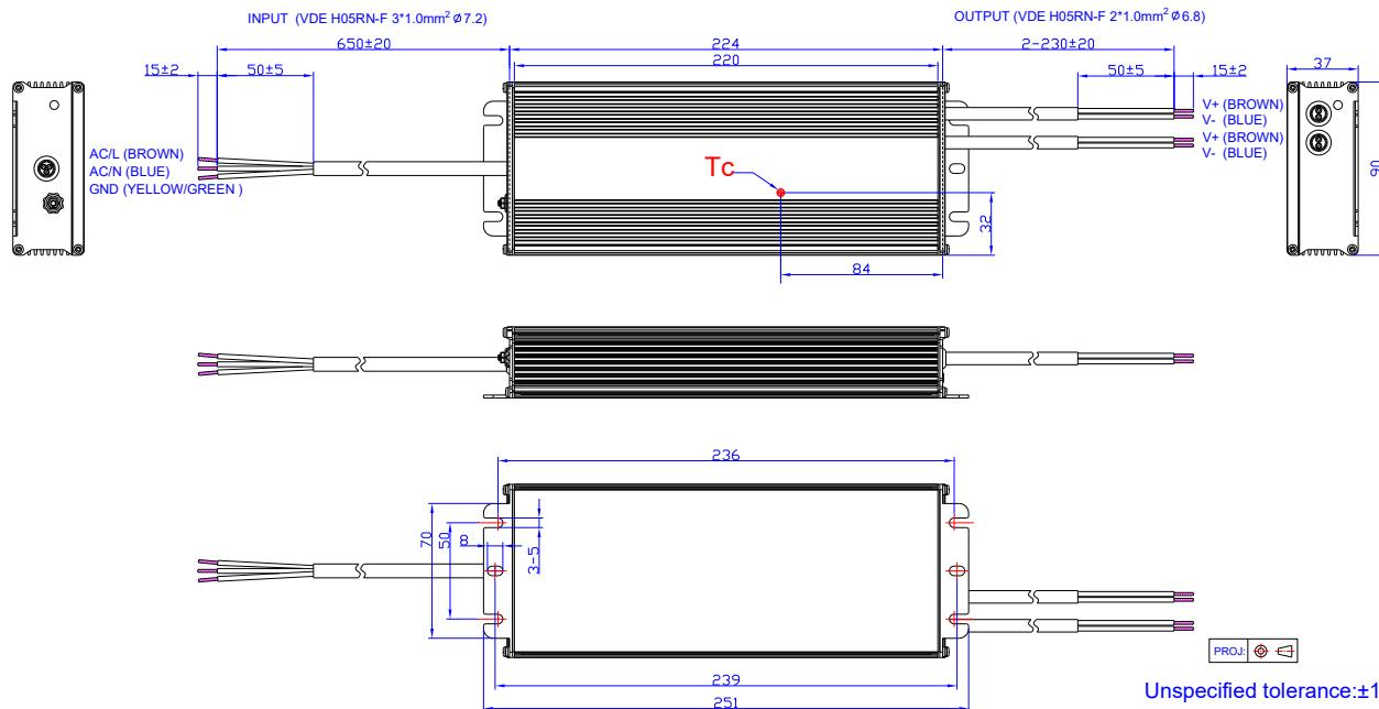
**Note:** The 2 DC output cables are connected in parallel internally because one 1.0mm<sup>2</sup> wire can only carry 10A. Please connect the 2 brown wires together and 2 blue wires together in application, or ensure each cable carries same current.
