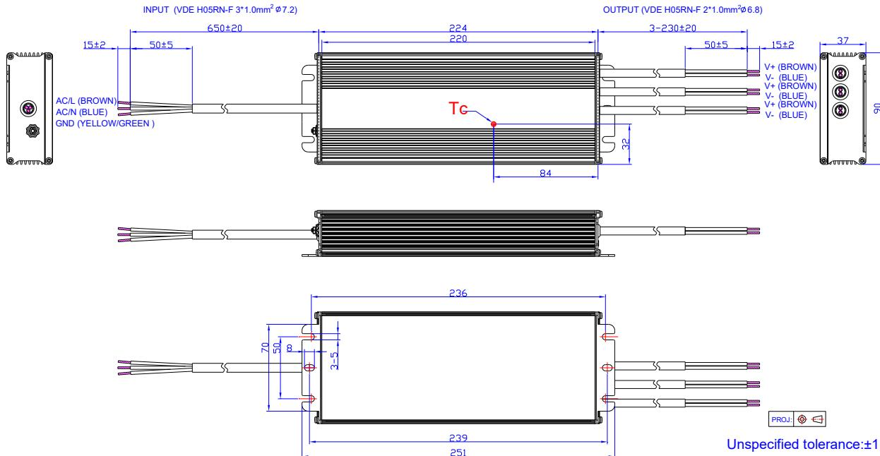
**Note:** The 3 DC output cables are connected in parallel internally because one 1.0mm<sup>2</sup> wire can only carry 10A. Please connect the 3 brown wires together and 3 blue wires together in application, or ensure each cable carries same current.
